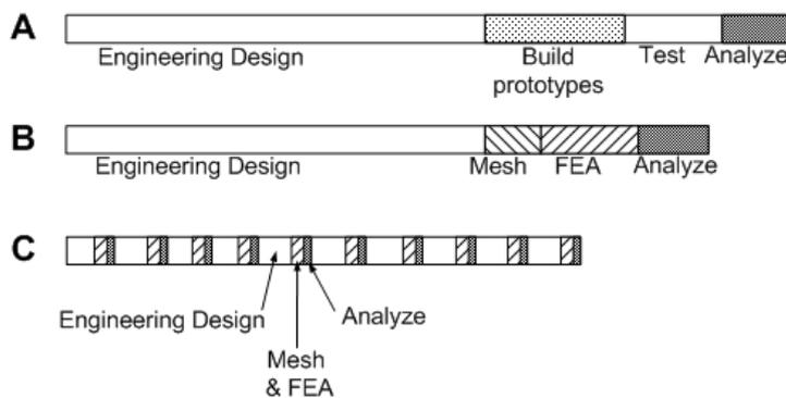
When CAD was introduced, CAD-drawings and later CAD-models were used for making test specimens. After some time it was realized that the models could be meshed and used for FEM analysis making the physical testing obsolete, case **B**. (This has not completely happened, and will never happen as long as legislation in many countries demands physical tests, such as crash tests).
